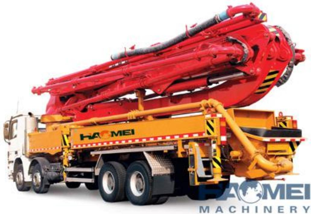
[Concrete pump truck](#) is also called [Concrete Boom Pump](#). The boom Pump allows quick setting-up by overcoming the necessity of cumbersome pipeline lying.
