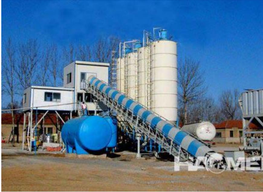
A [concrete batch plant](#), also known as a [concrete mixing plant](#), is equipment that combines various ingredients to form concrete. Some of these inputs include water, air, admixtures, act
